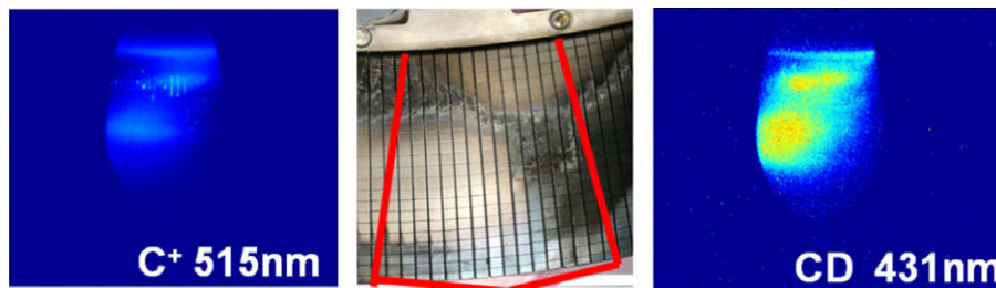
Fig. 4. CII and CD emission lines intensity distribution at the TPL surface. The central picture shows the field of view of the endoscope and the different zones discussed in this paper: erosion (shiny), thin deposits (bluish/black) and thick deposits (grey/looking coarse).
